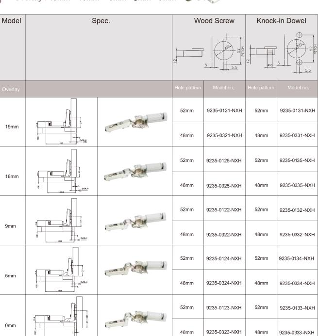
9236 Silent Snap-on Hinges For Thick Door 92°
