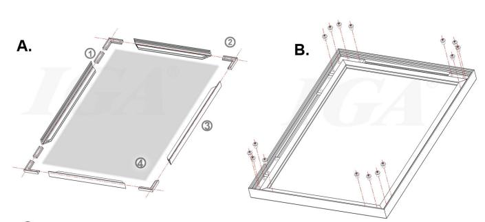
1.Fasten the frame with screws.
